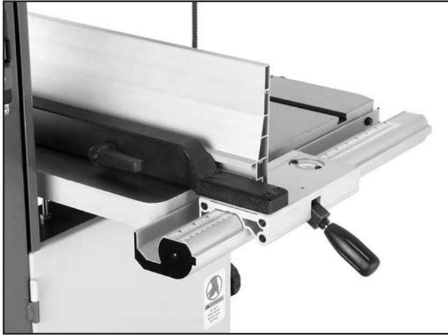
Figure 20. Correctly installed fence.
